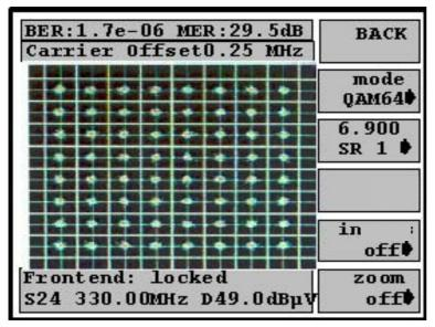
For digital transmission via cables, the modulation type QAM (Quadrature Amplitude Modulation) is used. The MSK 33 can represent the constellation of the modulation types, QAM64 and QAM128. For QAM 64, every 6 information bits are put together to one symbol and modulate one carrier in its amplitude and phase. With this, 64 conditions are possible, which a receiver must recognise for correct assessment of a QAM signal.
